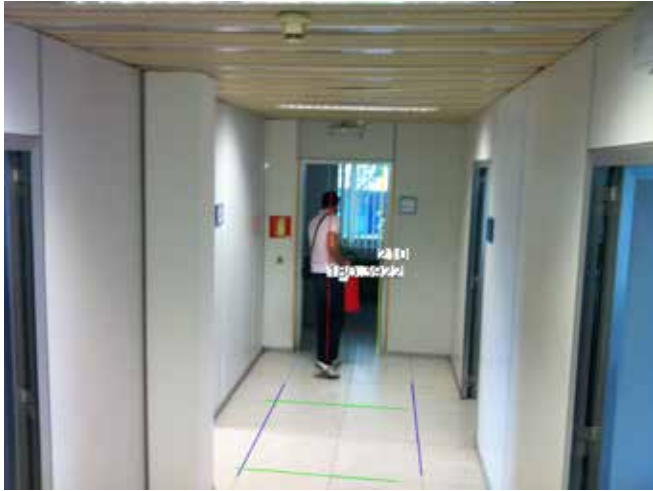
Figure 4: measurement of a subject with single view metrology
